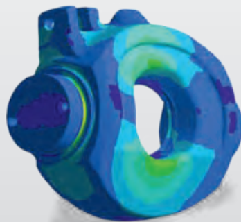
FE Analysis Stress analysis of swelling joint
